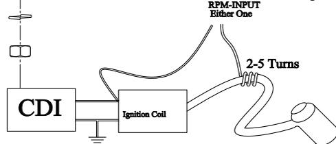
1. Signal intensity from ignition coil is dependent on vehicle type.
