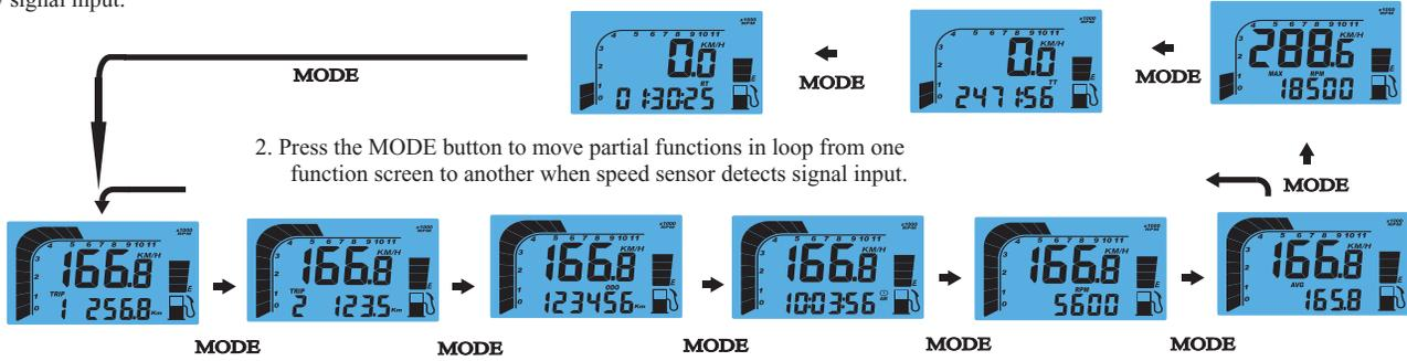
2. Press the MODE button to move partial functions in loop from one function screen to another when speed sensor detects signal input.
